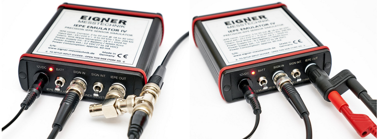
IEPE cabling: BNC T-piece
