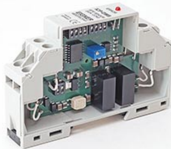
PCB mounting with position of the selector switches
